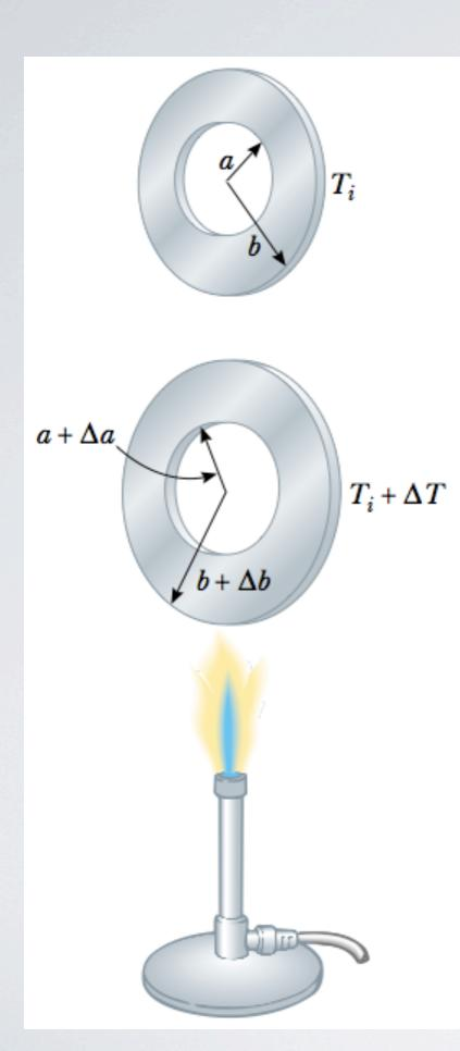
Thermal expansion of a homogeneous metal washer. As the washer is heated, all dimensions increase. (The expansion is exaggerated in this figure.)
